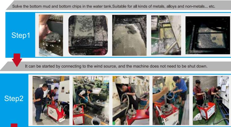
Vacuum negative pressure principle, easy drying, easy chip suction
