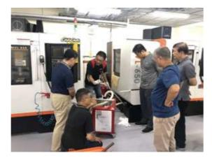
Double filter high efficiency purification and prolong liquid service life The highest filtering accuracy can correspond to 1um The processing machine can easily recover chips and bottom mud without stopping the machine
